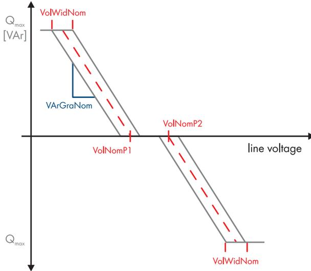
Figure 26: Characteristic curve for reducing reactive power with deadband and hysteresis
