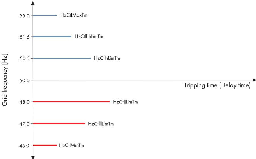
Figure 28: Tripping characteristics and time-dependant performance illustrated based on the frequency monitoring
