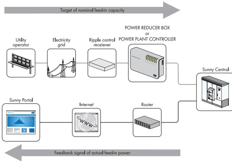
Figure 14: Principle of grid integration
