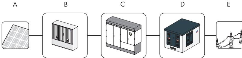
Figure 1: Principle of a grid-tied PV plant with an inverter
