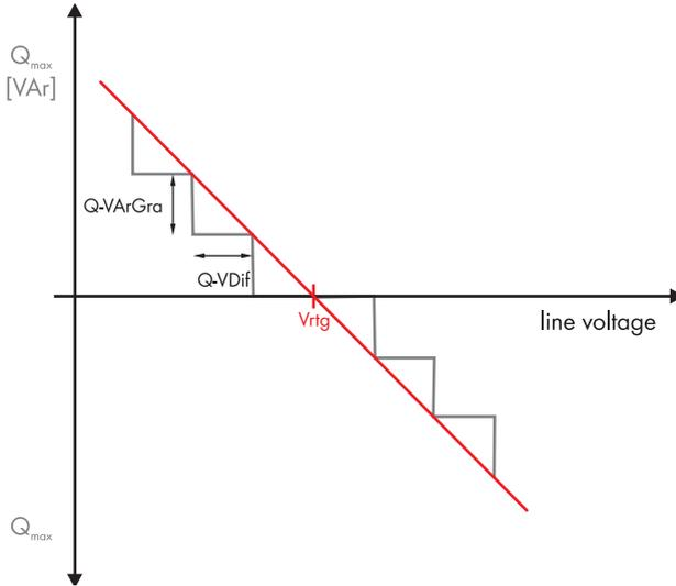
Figure 22: Characteristic curve for reducing reactive power dependent on line voltage
