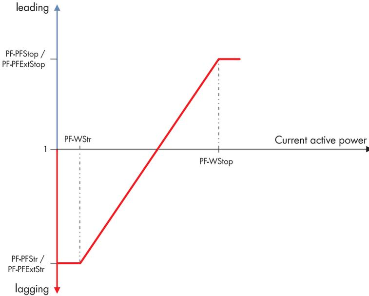
Figure 21: Characteristic curve for reducing reactive power dependent on active power
