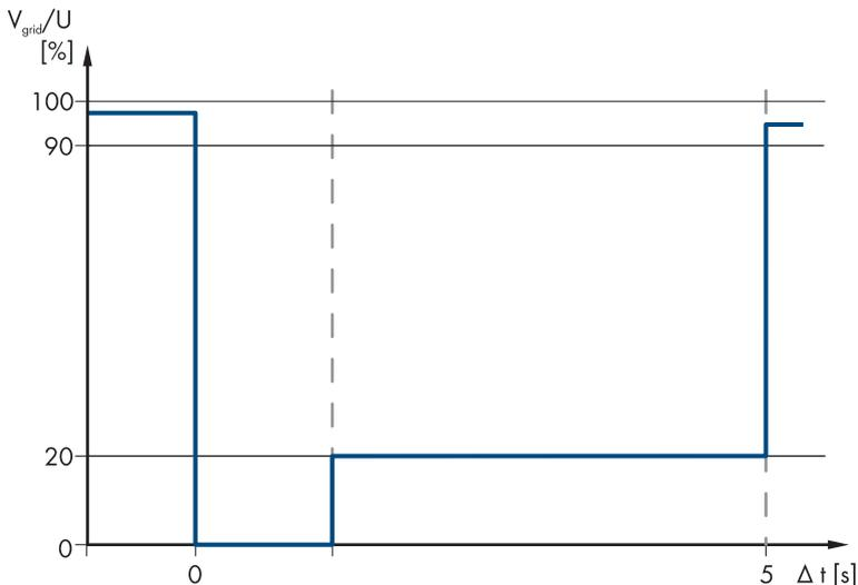
Figure 15: Maximum duration of voltage drop which the Sunny Central has experience without disconnecting from the grid
