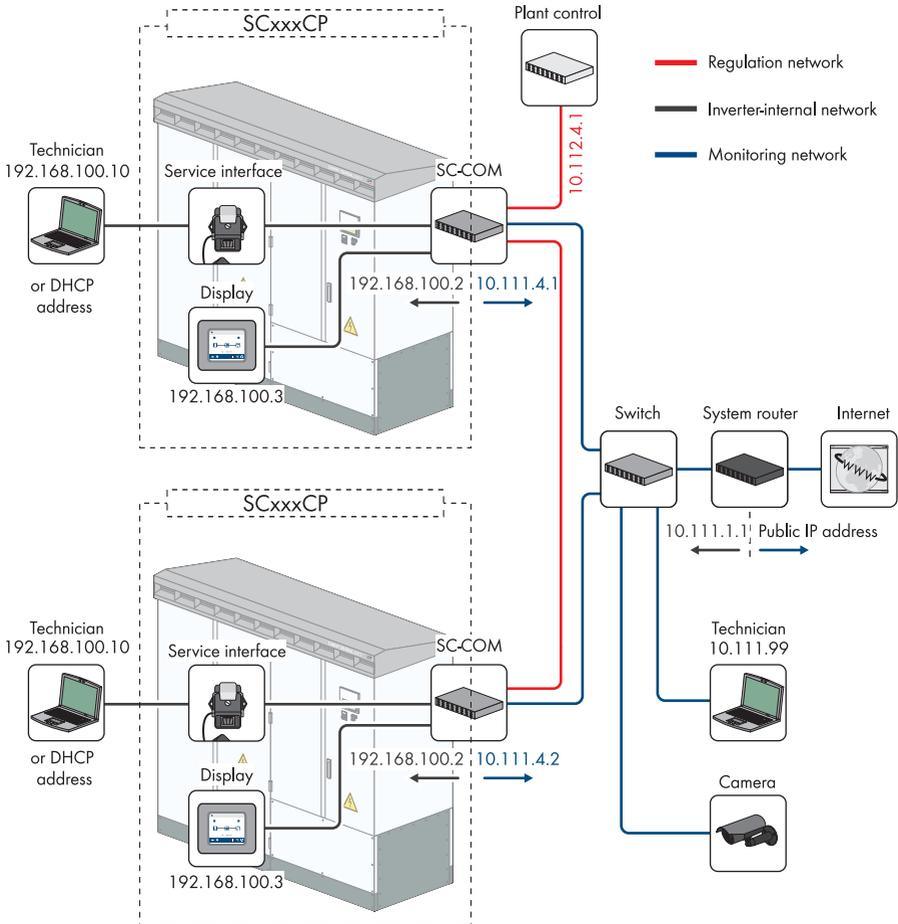
Figure 18: Example of a plant network of 2 inverters with indicator lights
