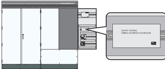
Figure 6: Sunny Central String-Monitor Controller
