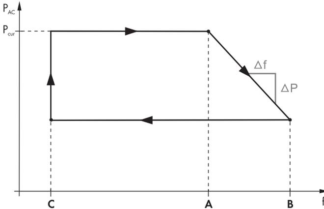
Figure 19: Behaviour of the Sunny Central when the P-HzStr frequency limit is exceeded
