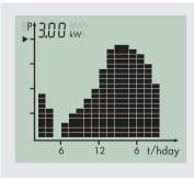
The inverter energy is shown as a diagram on the display. The daily graph is displayed by default. The right-hand flashing bar of the diagram represents the current hour. In case the inverter does not feed any power into the grid for a prolonged period (e.g. when the wind is calm), a gap is inserted into the graph. The bar for the current hour is updated automatically every five seconds. After four seconds, the bar goes off for one second and then displays the current value.
